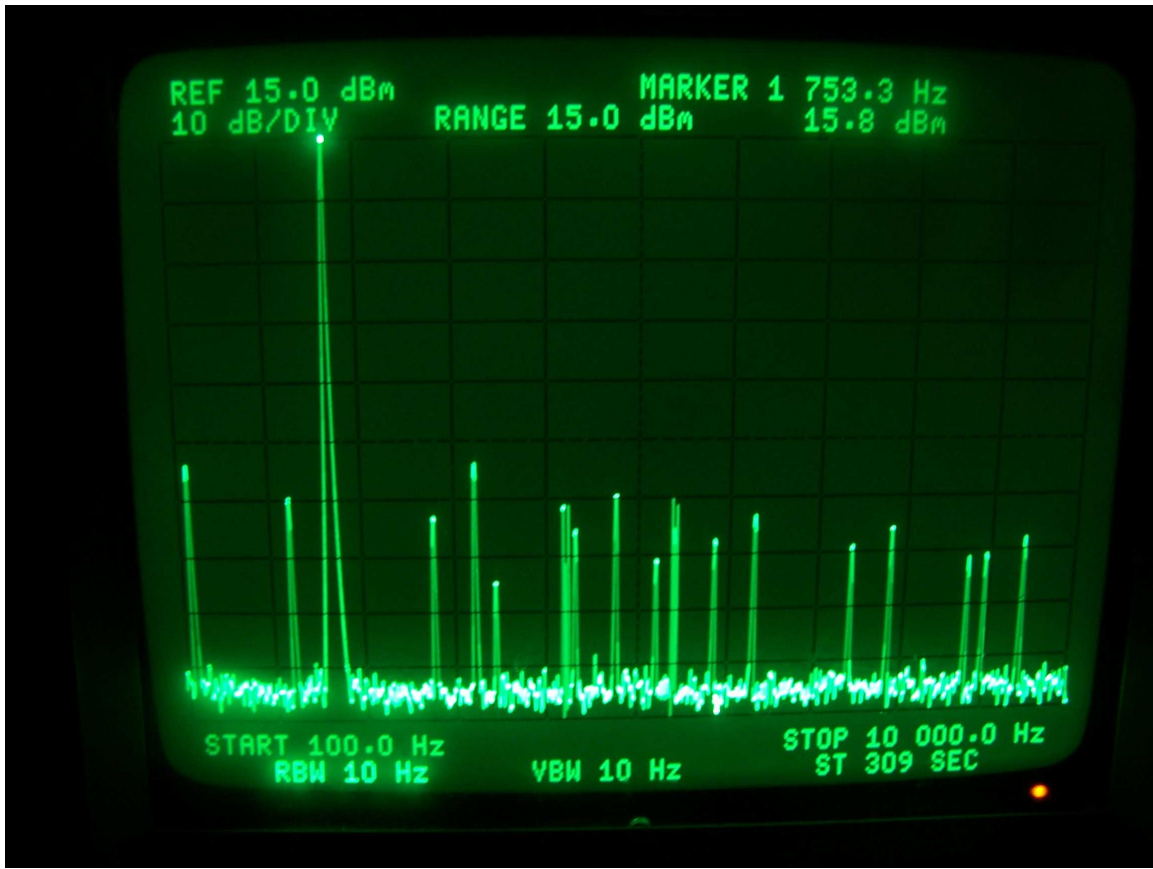
Figure 2: Response of DDS oscillator on lab board. Mid P/B was pushed.
