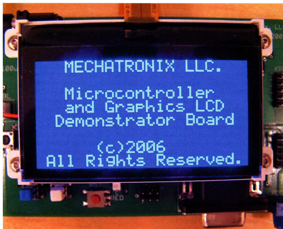
Figure 1: LCD controller in operation
